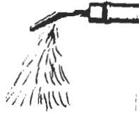
Spray Pattern with Insufficient Water
